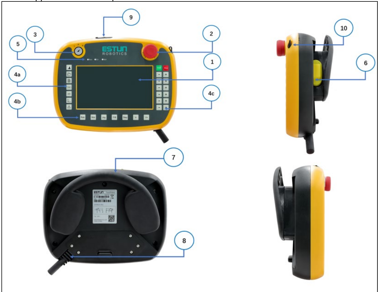
1. LCD display area; 2. Emergency-stop button; 3. Mode switch; 4. Keyboard area; 5. Indicator LED; 6. Enable switch; 7. Suspension bracket; 8. Cable connection area; 9. USB interface; 10. Operation pen
